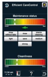
Efficient CareControl detects when the appliance needs to be cleaned. Efficient CareControl takes into account the individual cleaning behaviour and work routines such as longer breaks or the end of work.
