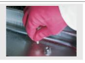
Place the moisturing nozzle in the descaling liquid and allow it to react (moisturing nozzle must be free of scale)
