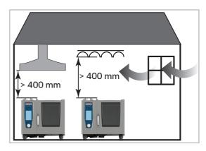
Room air-dependent gas furnaces with fans in front of burners without flow guards and total rated load in installation space less than or equal to 14kW. It is not mandatory that gas only be supplied to the burners when the exhaust system is in operation.
