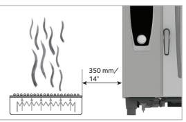
If it is not possible to keep the left side (or right, on 61 and 11) of the device a sufficient distance away from heat sources, a heat shield can reduce thermal loads.
