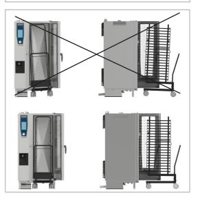
Make sure there is 200mm distance between the upper edge of the entry ramp and the floor with the unit feet.
