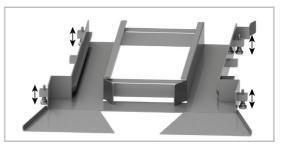
The entry ramp is attached to the right foot of the device using the ramp clamps.
