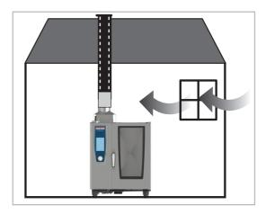
Fixed connection to a chimney is permitted if a flow guard is also in use.
