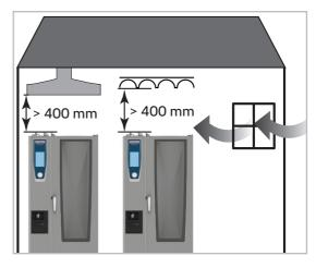
Room air-dependent gas furnaces with fans in front of burners without flow guards and total rated load in installation space greater than 14kW.
