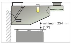
If steam from the ventilation pipe cannot be directed into an exhaust hood or a ventilating ceiling, there must be at least 500mm clearance space above the device.
