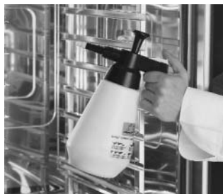
Spray the cooking cabinet with the special cleaner
