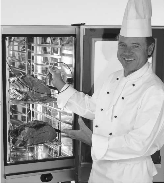
Using the core temperature cooking method you "can cook exact". Insert the sensor into the thickest part of the meat.
