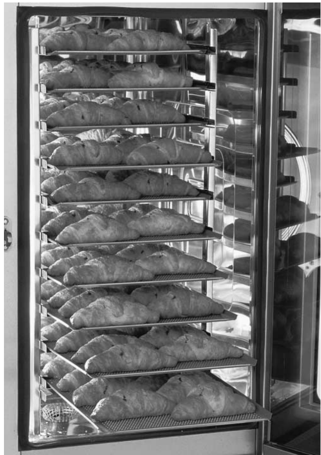
Perforated aluminium sheets conduct the heat quicker and evenly to the underside of the product.
