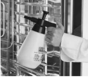
Spray the interior cabinet with the special cleaning detergent.
